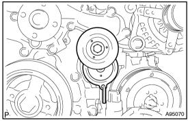
(b) While turning the belt tensioner counterclockwise, align its holes, and then insert the 5 mm bi-hexagon wrench into the holes to fix the belt tensioner.
